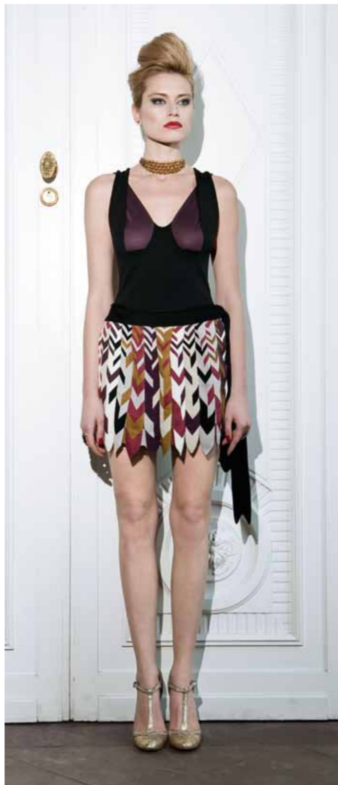
1110071 · CMS 530 HP · E 16 Fully Fashion top with shoulder straps, intarsia jersey structure, shaped by plating with lycra Knitting Time: 1 front piece: 20:48 min – 1,0 m/s
