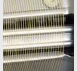
Fix coils separation: 1 mm
