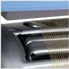
Yarn storage sensor (always maximum stock)
