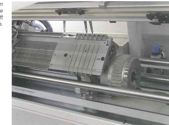
Cam box without cam carriage bridge allowing direct yarn feeding system, double systems cam boxes each with integrated bi-directional transfer.
