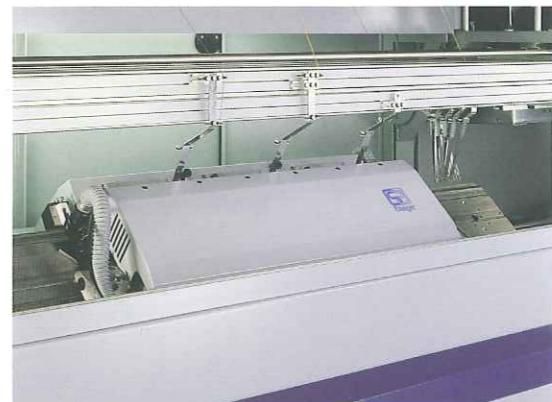
Carriage with 3 systems cam box optimises the production in general and especially in Intarsia for highest efficiency and cost savings.
