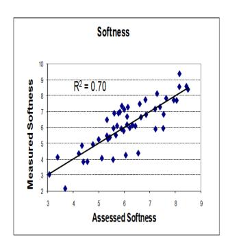
This figure to the left shows the level of agreement between the Wool HandleMeter (measured softness) and the expert panel (assessed softness) in judging the "Softness" of a series of 52 lightweight jersey fabrics.
