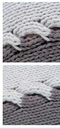
Two-color cable in two different gauges, knitted with one and the same machine.
