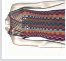
Intarsia rib dress with separate tubular starts for each color with 28 (30) intarsia yarn carriers, top part with smooth transition from the ribs into straps, indicated V-neck by ribs without intarsia binding.
