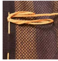
STOLL-devoiré knit®, STOLL-multi gauges® sleeveless Fully Fashion dress with fligree motif around the neckline, knitted with all needles, skirt part with rolled hem in plush and tubular structure with fligree motifs, knitted with all needles and 1 x 1 technique, top and skirt part combined with 1 x 1 tubular drawcord.
