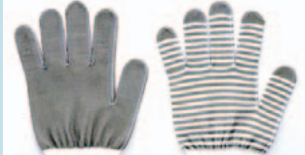
Left: Conductive yarn in every course Right: Conductive yarn every ten courses
